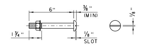
¾ " DIA A449 (TYPE I) ROUND HEAD BOLT (WITH WASHER AND PREVAILING TORQUE TYPE LOCK NUT) (SEE NOTE #8 ON S-360A) ONLY FULL DIAMETER BODY BOLTS WILL BE ALLOWED.
