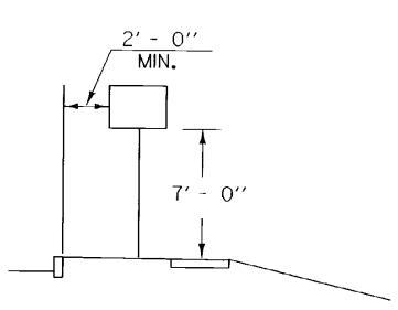
IF SUFFICIENT CLEARANCE IS NOT AVAILABLE BETWEEN CURB AND SIDEWALK MOUNT SIGN BEHIND SIDEWALK AS SHOWN AT TOP. CHECK FOR ADEQUATE R.O.W..
