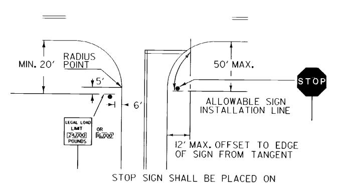
STOP SIGN SHALL BE PLACED ON DRIVERS RIGHT, MAINTAINING MAXIMUM VISIBLITY. CLEARANCE SHALL BE A MINIMUM OF 6' AND A MAXIMUM OF 50' FROM EDGE LINE OF INTERSECTING ROADWAY AND DOES NOT HAVE TO BE ADJACENT TO THE STOP BAR.
