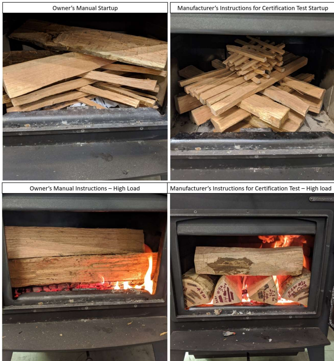
Figure 7. Fuel Loading Configuration – Stove 9
