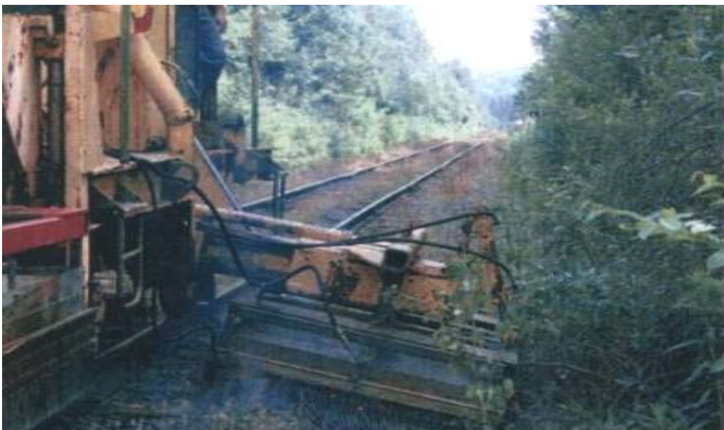
Figure 13: Thermal vegetation control equipment in action on the Saint Lawrence and Atlantic Railroad in Northeastern Vermont.
