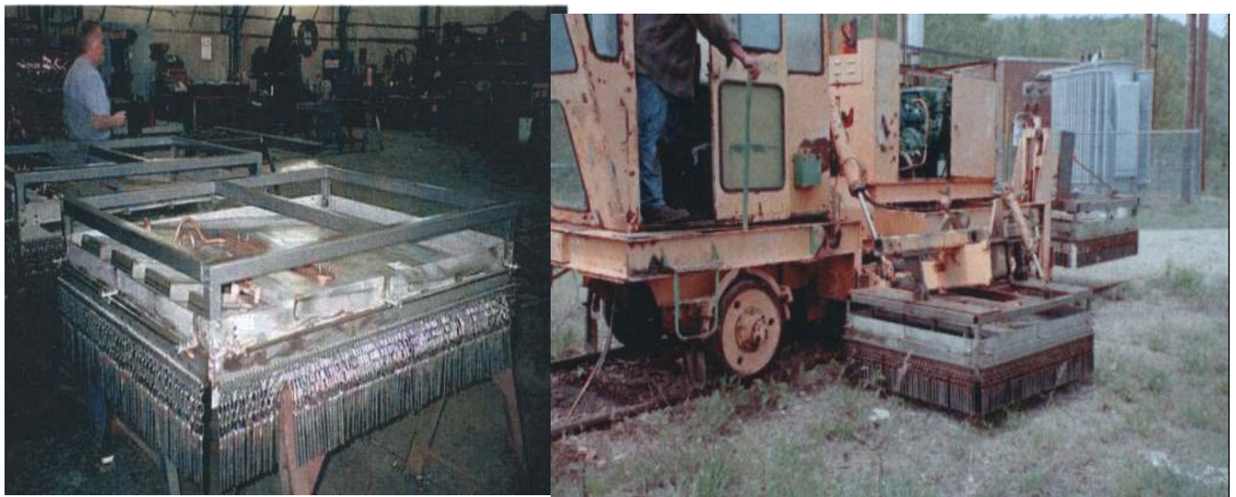
Figure 7: Infra-red units in the shop (left) and in the field (right)
