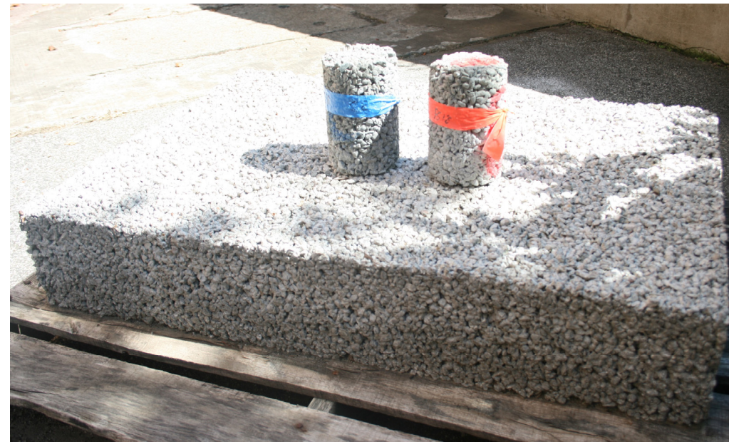
Figure 1 – PC samples used in testing on top of a pre-cast PC slab
