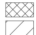
IMPERVIOUS AREA TREATED BY GRASS CHANNEL
