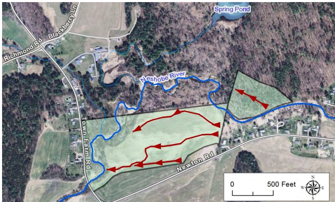
Figure 7: River corridor easement for parcels (shaded green) prone to flooding and erosion along the Neshobe River. Red arrows show the flow of water during extreme storms.
