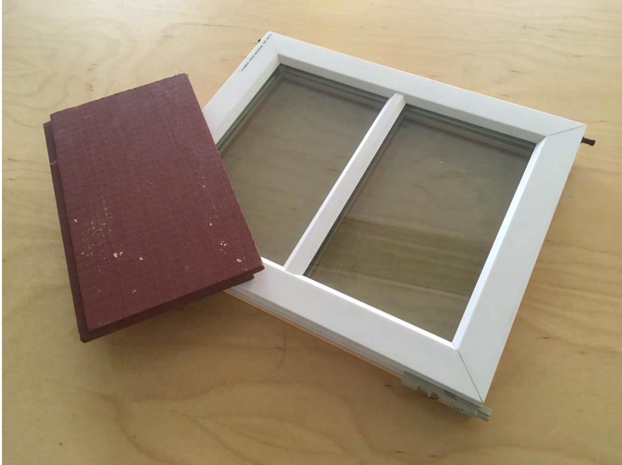
A typical simulated-divided-light, fiberglass-clad wood window and wood siding sample proposed for a new house in the village.
