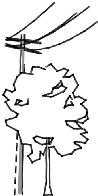
Figure 7. Trees Under Power lines - Select the appropriate tree with respect to mature height for under power or utility lines so it will not have to be pruned.
