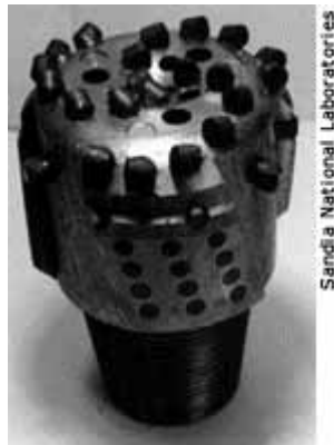
Diamond-studded drill bit developed at Sandia National Laboratories
