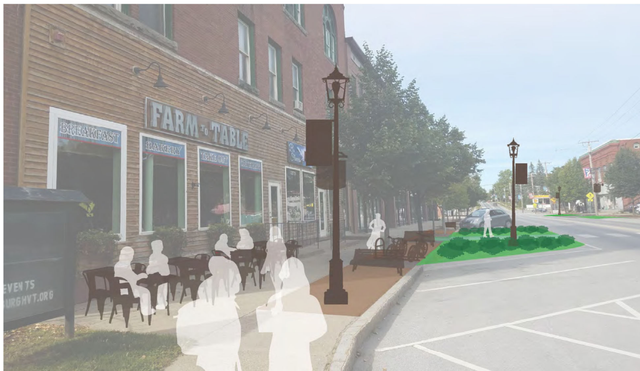
Rendering of a conceptual curb bump-out and other improvements to Main Street from the Vital Village Master Plan.
