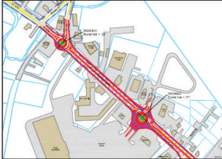
Suggested intersection improvements along the congested Route 7A/67A corridor include roundabouts at the intersection of those two highways and at the Monument Plaza intersection. (Northside Drive Roundabout Conceptual Design, 2006, by Resource Systems Group.)
