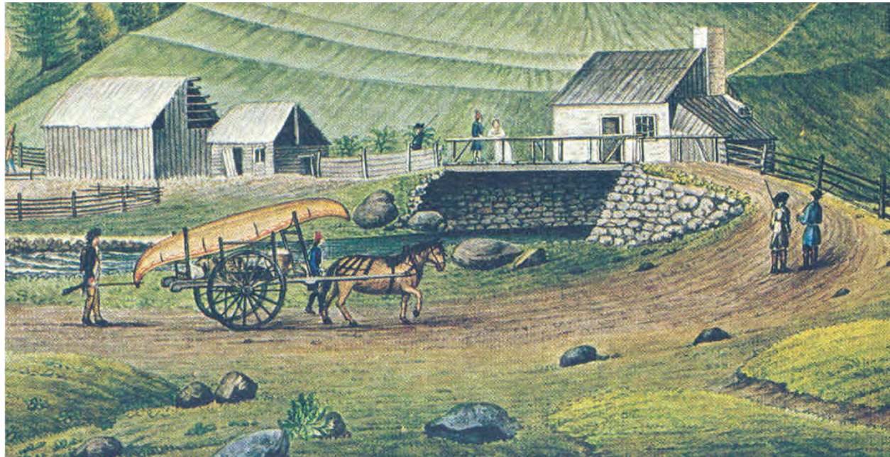
Thomas Davies watercolor, "A View of the Bridge on the River La Puce near Québec in Canada," 1788. Note both vertical and horizontal logs, or planks, used for buildings, in the style of en pieux ( poteaux ) debouts and poteaux en coulisse . Source: National Gallery of Canada.
