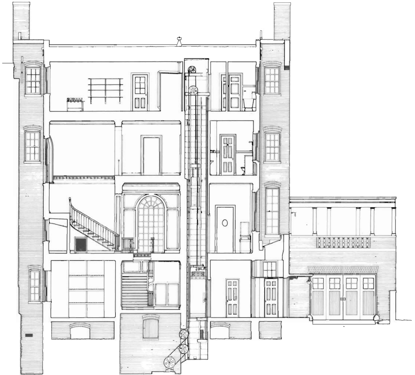
Woodrow Wilson House, District of Columbia (1915). The architect placed two exterior lightwells along the party walls of this house. They provide light to spaces that need light but not necessarily a view, such as stairwells, a pantry, a closet, bathrooms, and hallways. What appears to be a large arched window near the center of the drawing is actually a borrow light illuminating the stair landing between the first and second floors.
