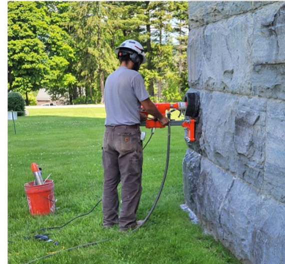
Goodman Jack test to evaluate stone's reaction to stress
