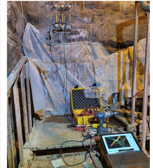
Deformability testing measuring stiffness & stress-response of stone
