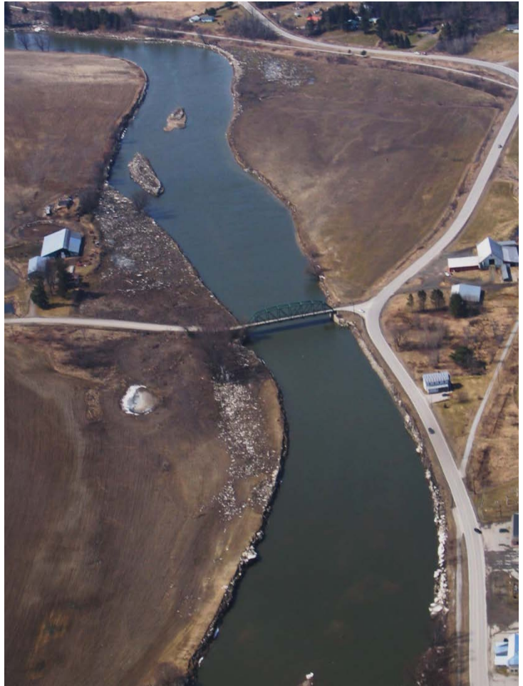
Figure 11: Missisquoi River flooding at low spot on Boston Post Road looking downstream. Note the ice chunks on the floodplain indicating recent flood flow locations (Source: Staci Pomeroy, ANR, March 29, 2006)
