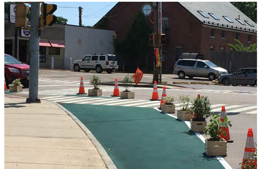
Top: Locally-made wooden crates in Burlington, VT (Street Plans); Bottom: store bought crates used to define the edge of a curb extension in Portsmouth, NH (Street Plans).
